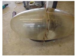
• Mark pants for final trimming at tire and gear leg. 3/8"-1/2" clearance all around tire and 1/8"-3/16" around gear leg and rubber.
