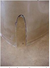
• Trial fit the aft sections to the plane. Open up the tire hole a little at a time as needed. This varies with the brand of tire you have.
