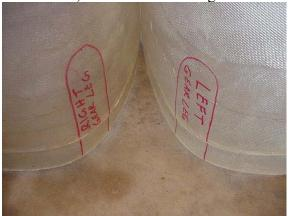
• On each aft section mark the outboard tire scribe line with a sharpie. Note that the wheels and tires favor the outside of the wheel pant. The inboard part of the pant covers the gear leg and brake
