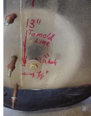
• Remove the 10-32 forward 2 inboard mount screws. Fit the fwd sections onto the aft ones. Trim tire hole and aft edge as needed to get a good fit. Tape in place with masking tape.
