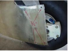
• Drill outboard mounting hole to match hole in the center of the axle stub with ¼" drill. Take care not to damage the threads in the axle stub. This hole should be approx 13" from the center mold line and 7/8" aft of step joint as shown. Install a ¼-28 bolt in the outboard hole.
