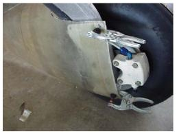
• Check for ½" min clearance between the top of the tire and inside of aft section. Use a small block of wood to hold this spacing.
