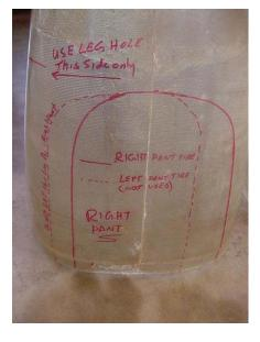
• Mark matching outboard tire scribe lines on the fwd sections one left one right.
