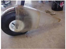
• When adequately trimmed, the pant should have 2 ½" of clearance to the floor at the extreme aft end and the step at the front end should fit to the brackets as shown. Also check that they aligned to the airplane center line. Do this by looking at the tire tread and the mold line on the aft sections.
